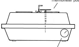
Hygrometer position TO USE AS A HYGROMETER IN A HOVA-BATOR
