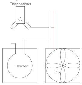
This wiring diagram is an option for those who would like the fan to turn off when the heater turns off.
