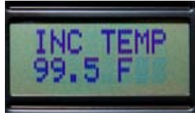
INC TEMP - Shows actual temperature inside incubator.
