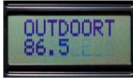
OUTDOORT - Shows temperature outside of incubator.
