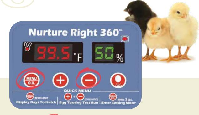
PRESS AND HOLD THE "MENU" AND "-" BUTTONS SIMULTANEOUSLY FOR AROUND 5 SECONDS. THE INCUBATOR WILL BEEP, AND THE DISPLAY WILL BLINK ONE TIME, INDICATING THAT THE INCUBATOR HAS SUCCESSFULLY BEEN RESET.
