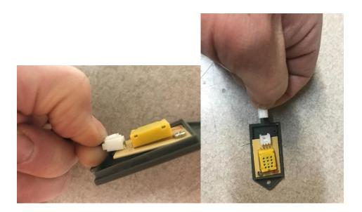
3. Separate the housing on the replacement sensor and reattach the white clip to the port. Reconnect the sensor casing and start up your HumidKit.
