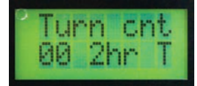
TURN CNT - Shows amount of times the turner has turned. Resets at 1000. No count on hatcher models.
