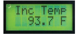
INC TEMP - Shows actual temperature inside incubator.
